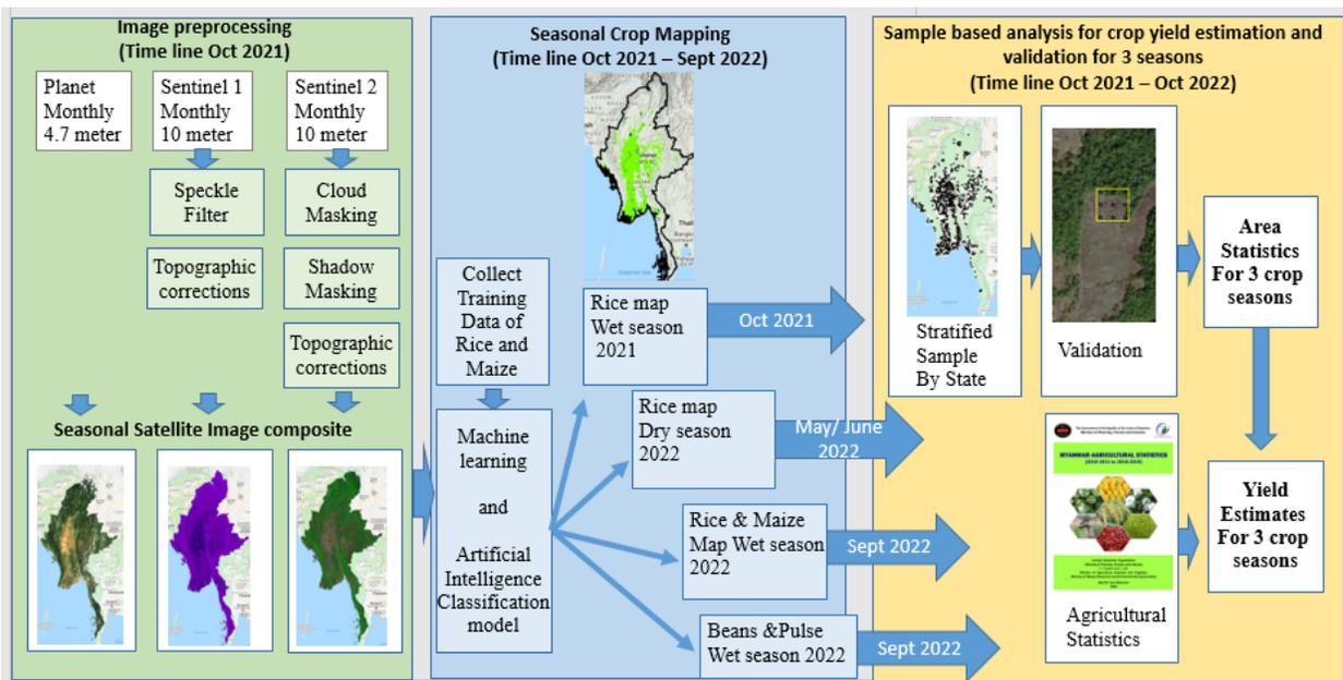
Figure 2. An overview of the satellite image processing (left), the machine learning approach (middle), and the data validation (right) to estimate the crop production per state and region.
